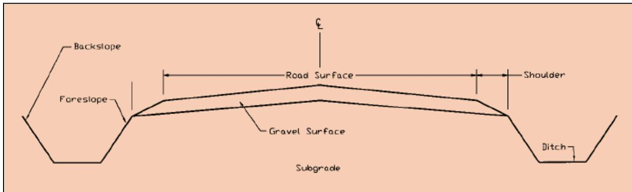
Figure 3-1: Road cross section (from *Gravel Roads and Maintenance and Design, SD LTAP Nov. 2000*)
