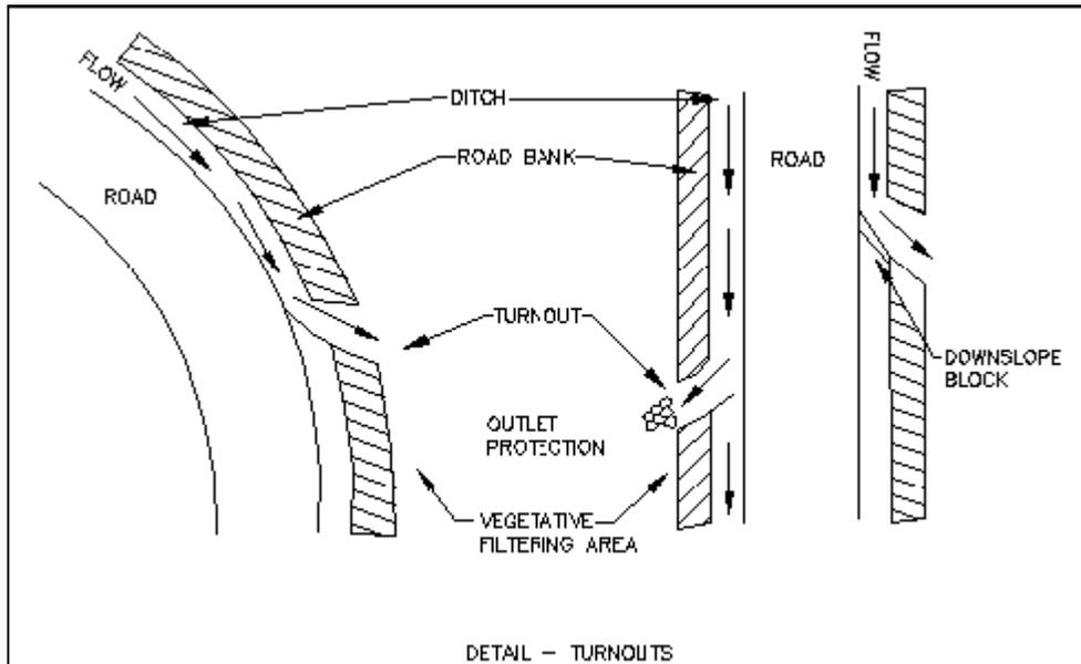
Figure 2-3. Typical Locations for "Turnouts" ("Tail Ditches") (from Recommended Practices Manual, A Guideline for Maintenance and Service of Unpaved Roads, February 2000)
