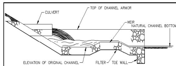
Figure 4-2. Weir-formed Plunge Basin (from
