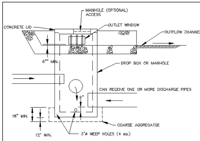
Figure 4-5. Stilling Well Illustration (from Recommended Practices Manual, A Guideline for Maintenance and Service of Unpaved Roads, February 2000)
