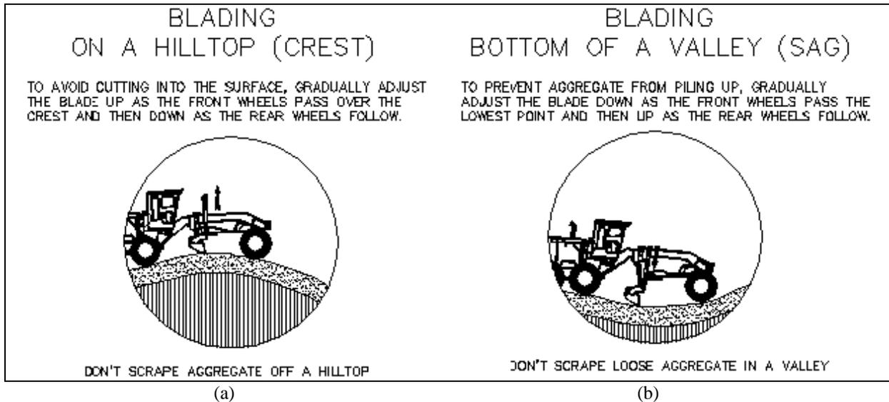
Figure 1-3. Blading on Hill Crests and in Valleys or Swags (from Recommended Practices Manual, A Guideline for Maintenance and Service of Unpaved Roads, February 2000)
