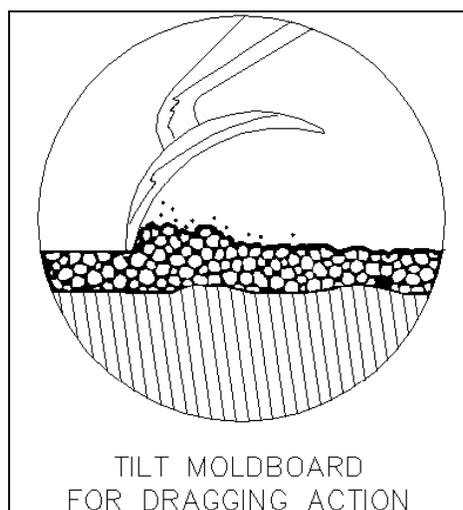
Figure 3-1. Blading (from Recommended Practices Manual, A Guideline for Maintenance and Service of Unpaved Roads, February 2000)
