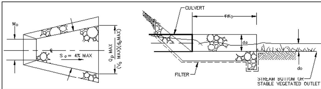
Figure 4-3. Splash Apron (from Recommended Practices Manual, A Guideline for Maintenance and Service of Unpaved Roads, February 2000)
