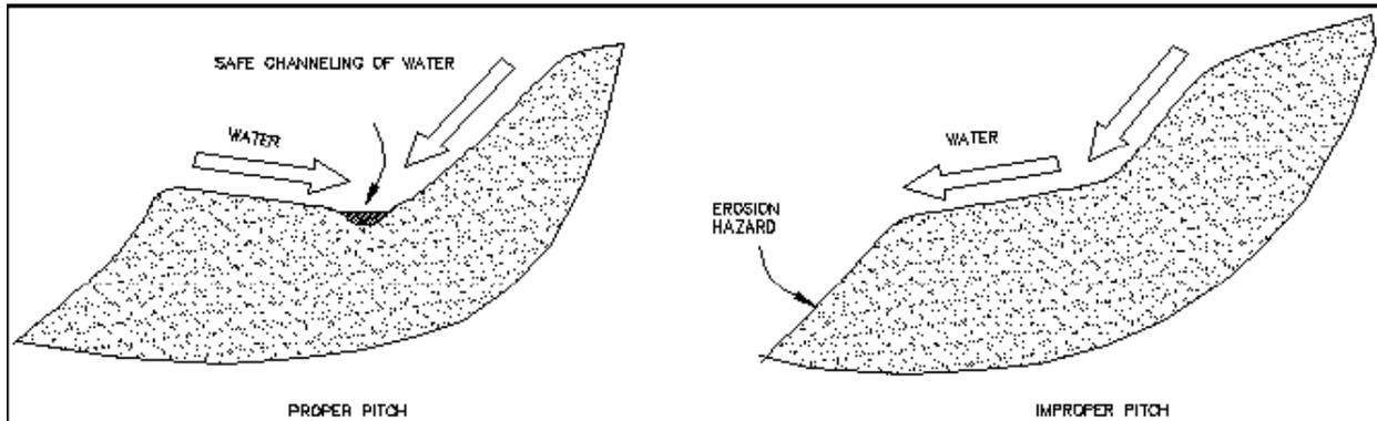
Figure 2-1. Hillside Pitch of Roadway and Proper Ditch Location (from Recommended Practices Manual, A Guideline for Maintenance and Service of Unpaved Roads, February 2000)
