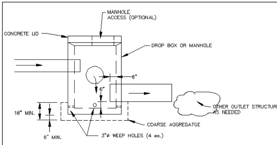
Figure 4-4. Drop Inlet/Box/Manhole Illustration (from Recommended Practices Manual, A Guideline for Maintenance and Service of Unpaved Roads, February 2000)
