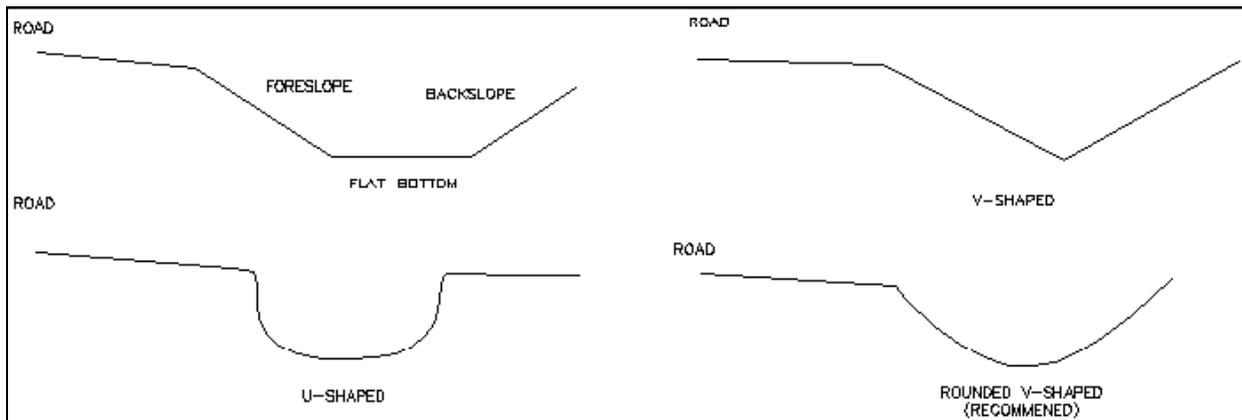
Figure 2-2. Common Ditch Shapes (from Recommended Practices Manual, A Guideline for Maintenance and Service of Unpaved Roads, February 2000)
