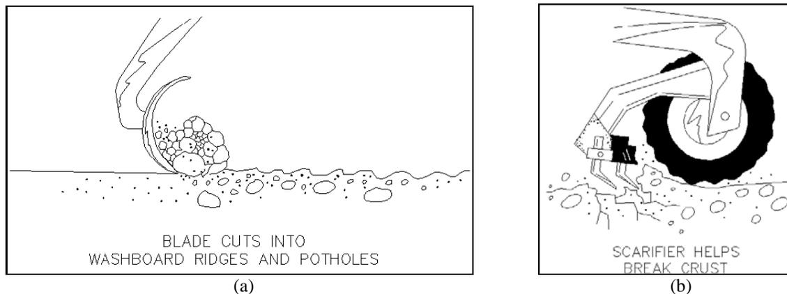
Figure 1-4. Grading Tools (from Recommended Practices Manual, A Guideline for Maintenance and Service of Unpaved Roads, February 2000)
