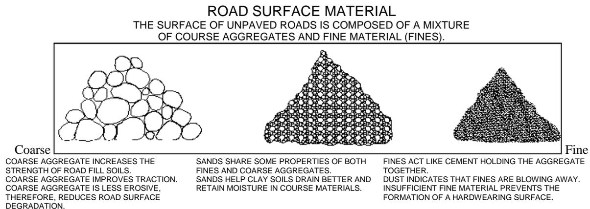
Figure 1-6. Aggregate Comparison (from Recommended Practices Manual, A Guideline for Maintenance and Service of Unpaved Roads, February 2000)
