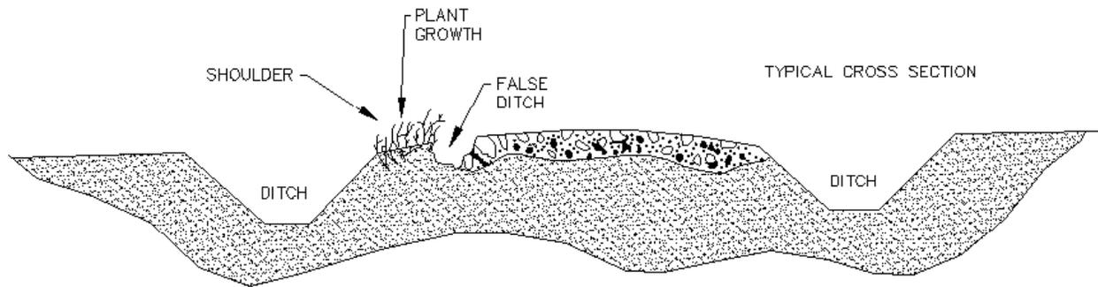
Figure 1-5. False Ditch (from Recommended Practices Manual, A Guideline for Maintenance and Service of Unpaved Roads, February 2000)
